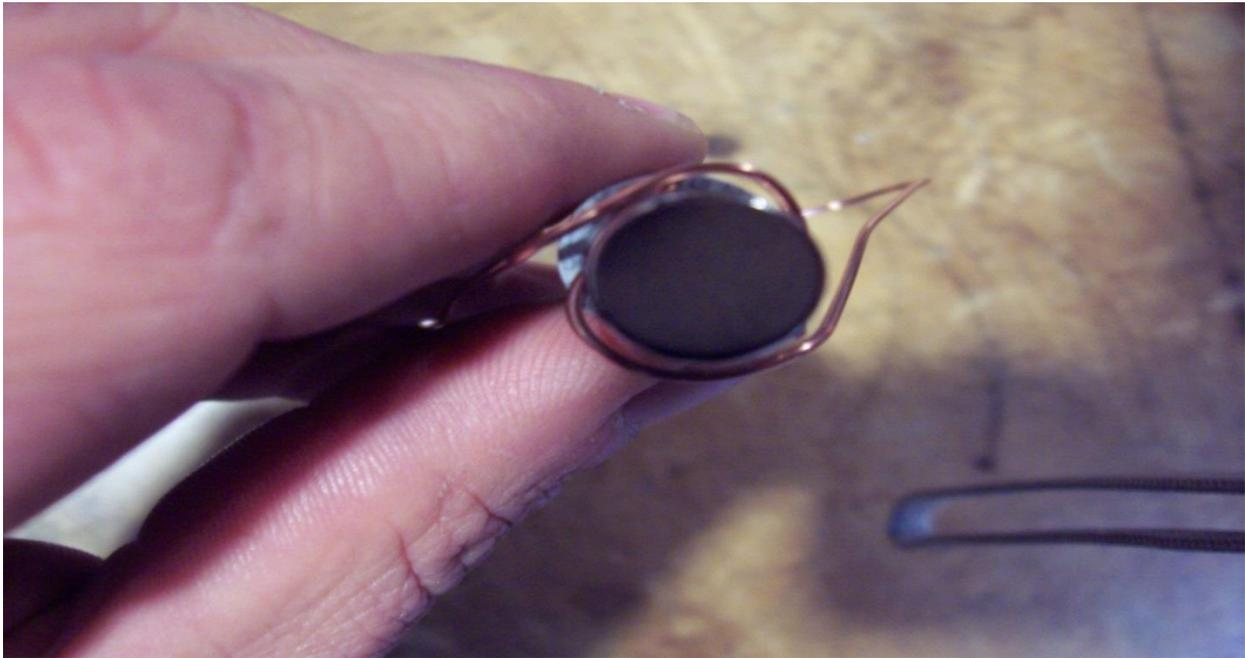
The wire should wrap around the magnet, the two ends should not touch. You do not want this to be too tight or the heart will fail to spin.
