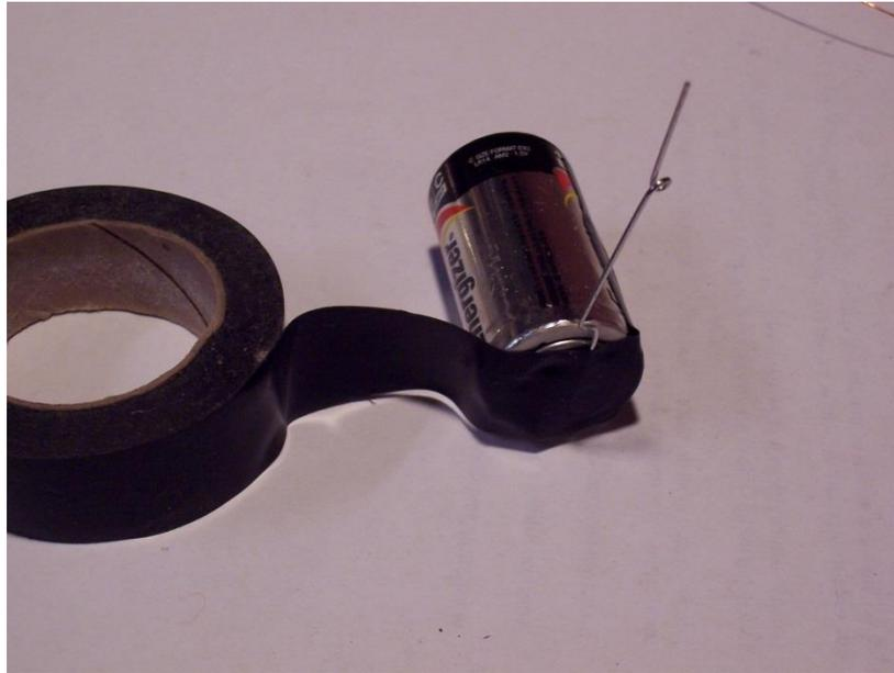
Make the clip wider to fit around the (+) positive post of the battery.
